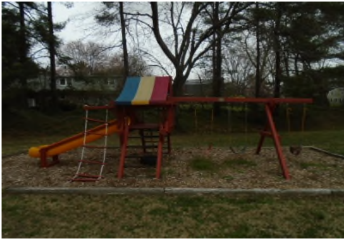
Tot-lots need replacement at end of life and fill replenishment every 2-years-children falling on non-absorbing material causes 70% of tot-lot injuries. Equipment cost will vary with features desired. Funding for mulch replenishment is from the operating account and is not included in the reserves.
