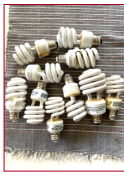
CFL light bulbs These bulbs contain mercury, and do not go in the regular trash.
